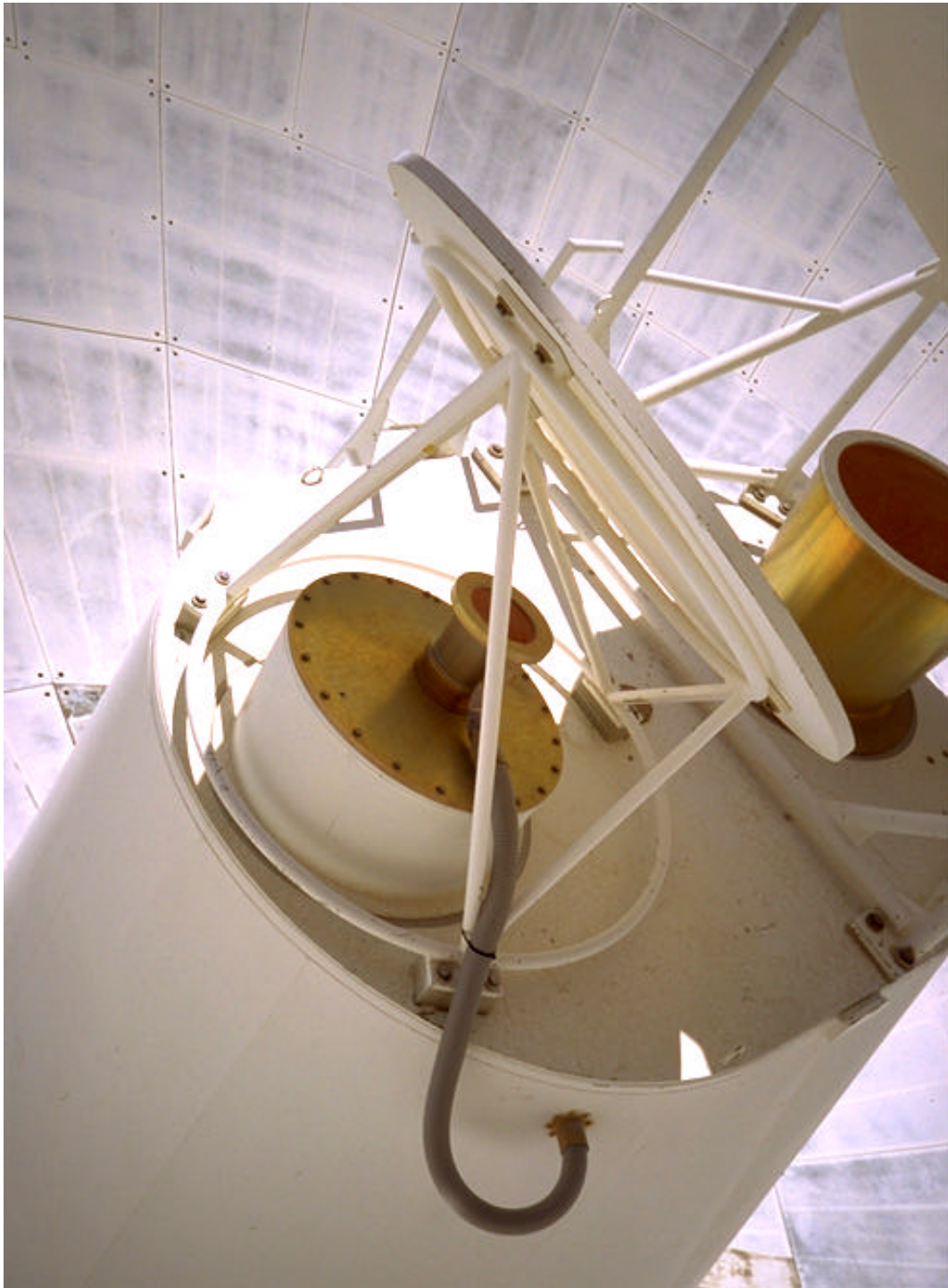
In the center of the picture is the top of the X-band feed horn. To the right, is the S-band feed horn. The “J” shaped hose coming out of the cone and running to the top of the feed is the X-band rain blower hose.
