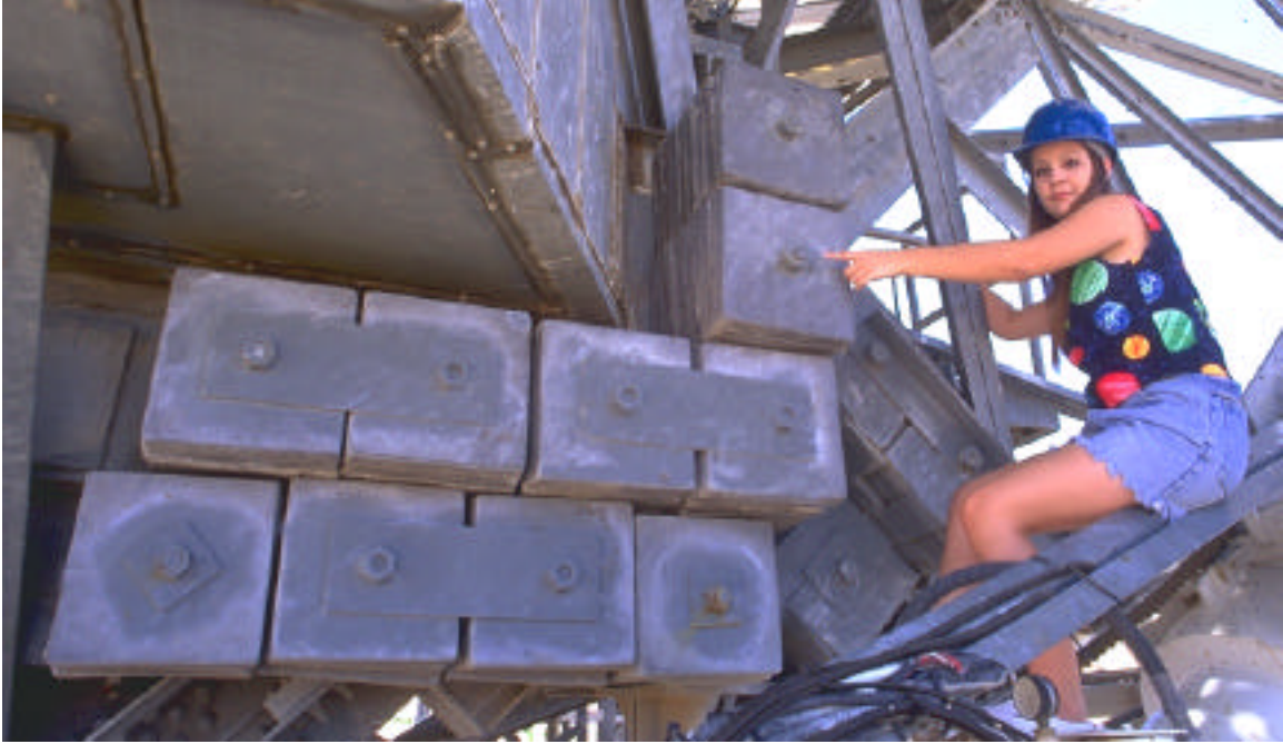
I'm pointing out the declination carriage counter weights. Each one weighs approximately 100 pounds.
